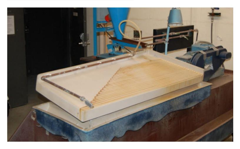
The Wilfley Tables are gravity concentrating devices that separate based upon differing densities of the material. They are effective in concentrating high density minerals, such as
