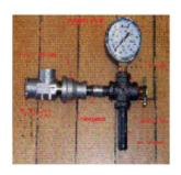
At left, the pressure relief valve furnished with the stainless steel pressure filter, and assorted fittings and pressure gauge
