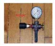
At left, the pressure relief valve furnished with the mild steel pressure filter, and assorted fittings and pressure gauge
